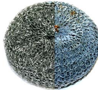
KnitMesh scourer before and after corrosion testing
